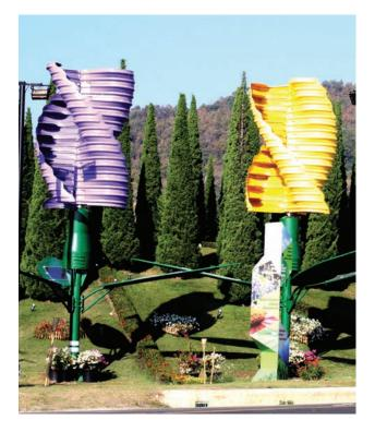
● A power-generating tree, consists of an advanced vertical-axis windmill and 3 photo-voltaic solar panels, is an alternative energy source. Visitors can appreciate such an environmental-friendly product specifically designed to suit Thailand's strong sunlight and low wind. Working system of power-generating tree obtains energy through the conversion of wind movements and sunlight into electricity, which is charged into a system of batteries for later use.
